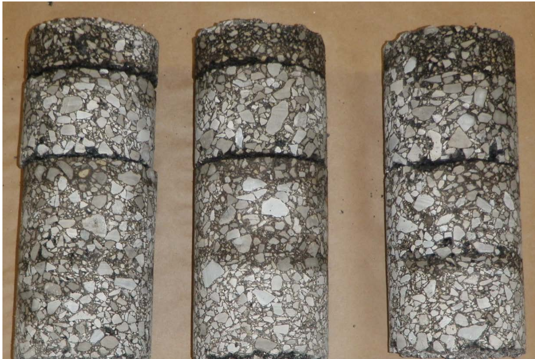
Figure 3. Cores showing layer debonding from Missouri.
