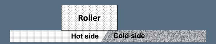
Concern with this method is if insufficient HMA laid on hot side at joint, then bridging occurs with first pass (roller supported by cold mat)
