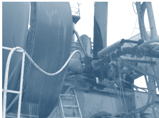
Figure 35. DAT injection point.
