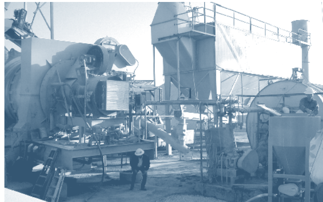
Figure 27. Pneumatic feeder (right) for drum plant. (38)
