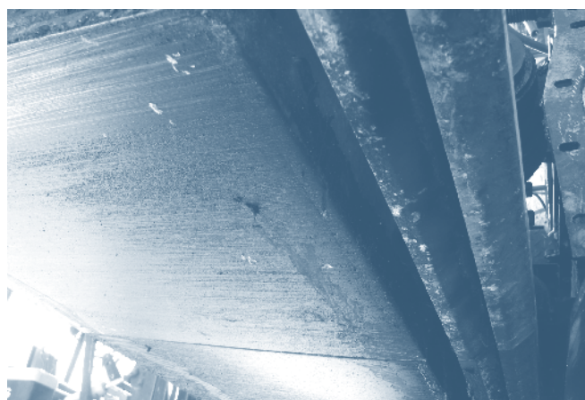
Figure 18. Close-up of tamping bars and vibratory screed.
