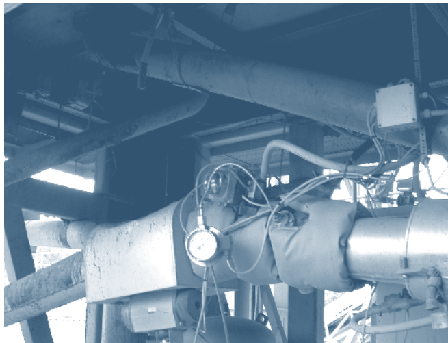
Figure 33. Asphalt line, expansion chamber, controls, and transfer pipe for foaming hard asphalt.
