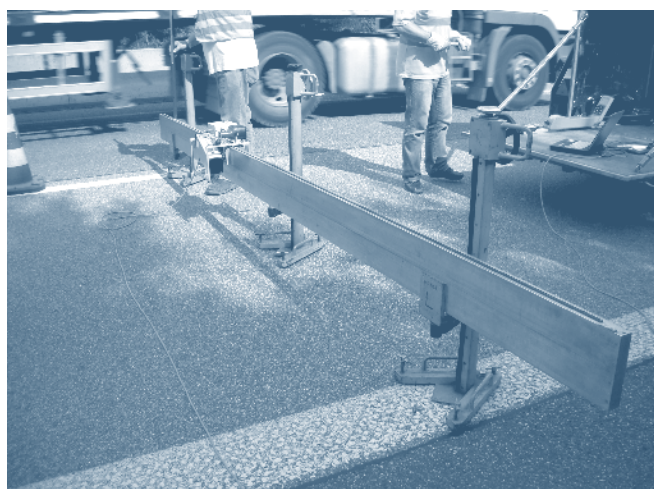
Figure 6. Transverse profile measurements.
