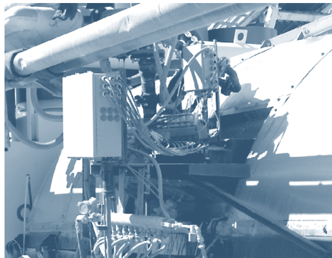
Figure 37. Astec multinozzle foaming manifold. (40)
