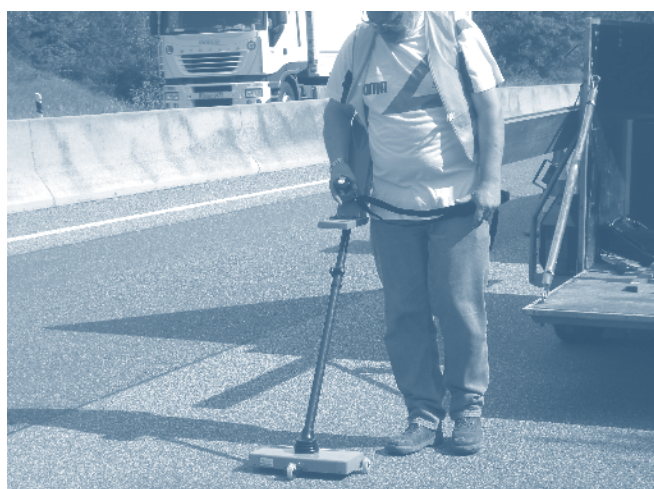
Figure 7. Layer thickness measurements.
