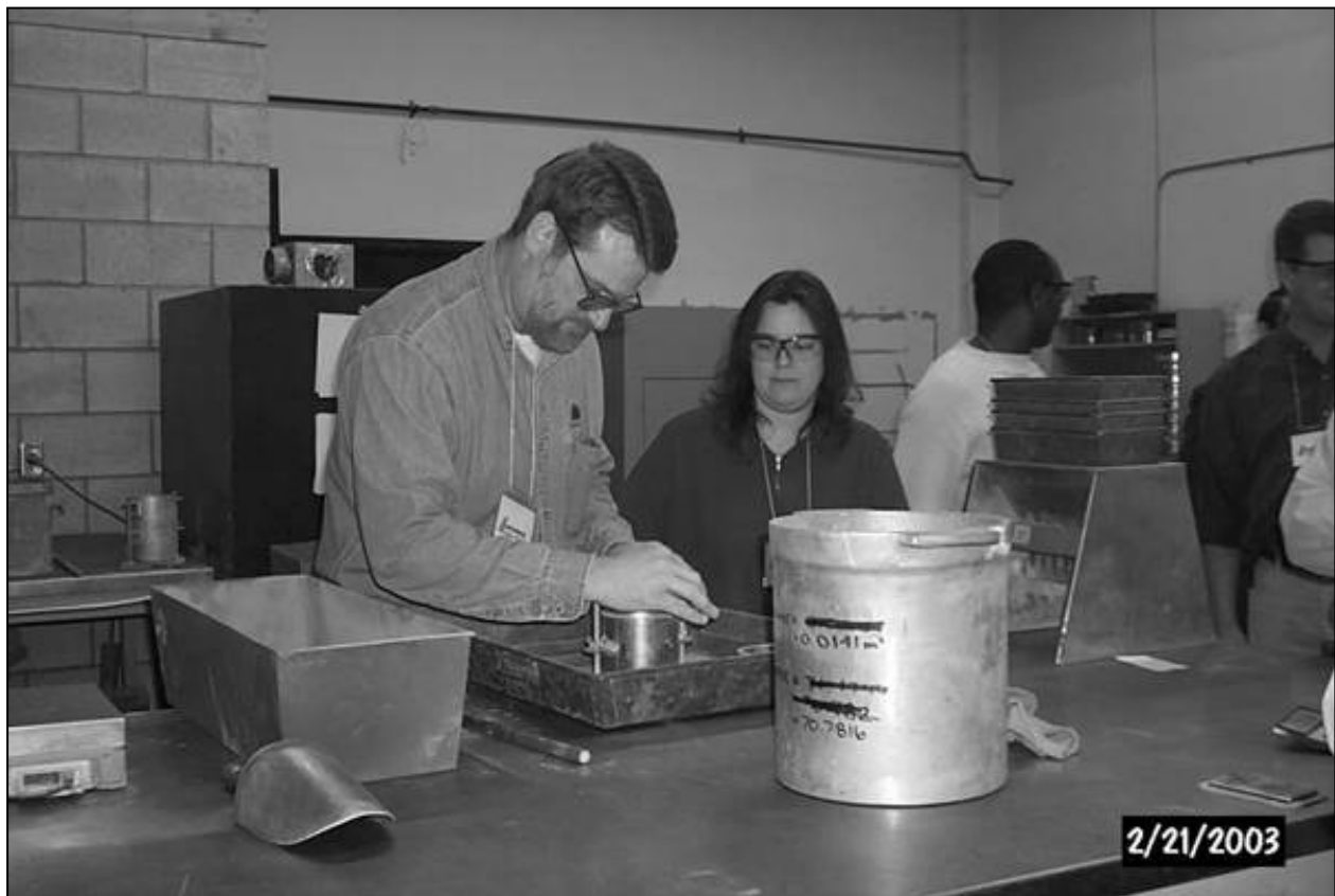
Photograph 1. Bill Pine in Action - Demonstrates Fine Aggregate Unit Weight Test at the First Bailey Course Held in Ontario
