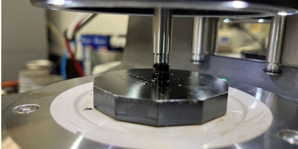
Figure 4. DSR testing using the 8-mm parallel plate measurement geometry
