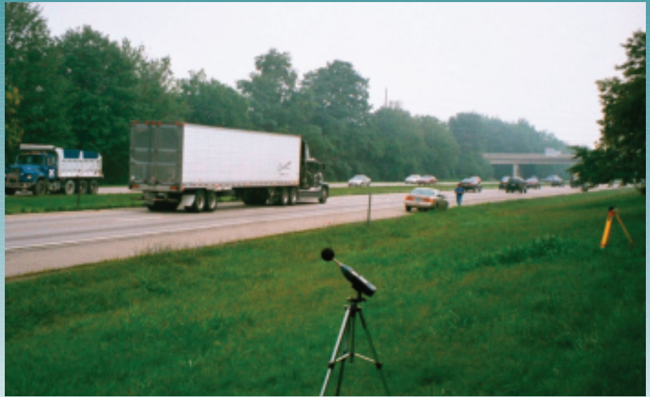
A 4–6 decibel reduction in noise was measured after placing a HMA overlay over the existing PCC pavement.
