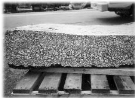
The plastic mix below the SMA course showed signs of serious deflection.
